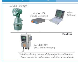
A single unit of model HDM or a combination of model HDM enables a use of Model HGC303 system in single or multi stream pipeline metering application \*1 and process application \*2 such as turbine control for power plant and heat value monitoring for industrial automation.
